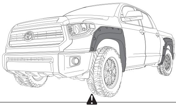
WARNING!! Do not install Hood Scoops or other Body Parts directly Over Wrapped areas. Before installation of the parts, you must leave at least a 1/4" (6mm) perimetral clearance "Free from Vinyl" surrounding the part, before Part installation.
